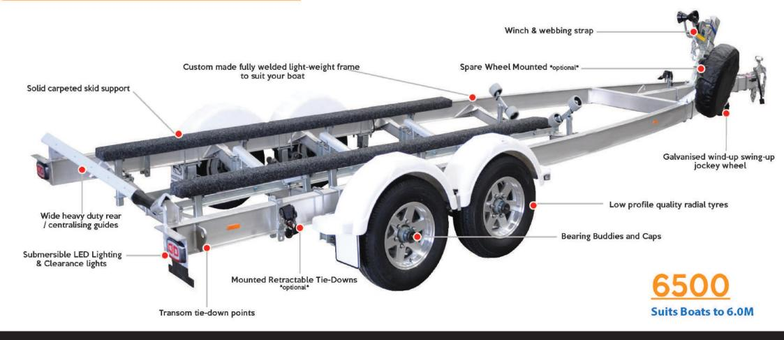
The AL Series is standard with skid pads and optioned with rollers and/or teflon skids. Some photos may include optional extras or change in design
