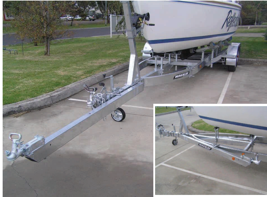
Swing Around Drawbar - Gain an EXTRA 2M
